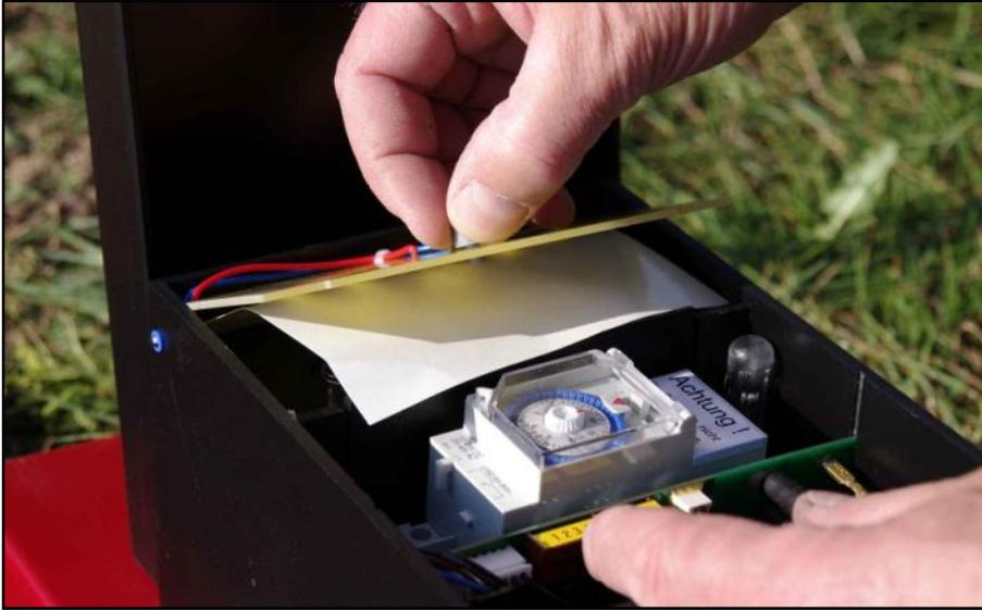
Open the lid from the electronic unit (108510). Lift the battery contact board and remove the paper strip to contact the batteries with the board. After removing the paper strip press the battery contact board back down to close it.
