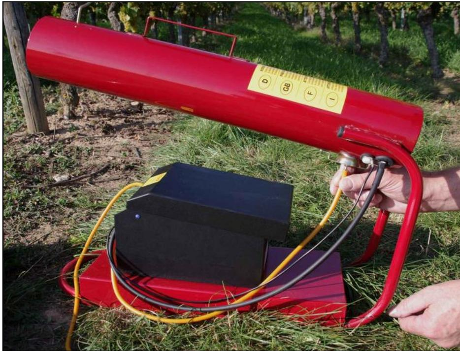
Once the propane nozzle is screwed in, push the gas hose onto the nozzle.
