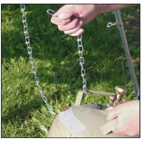
Hang one side of the chain (102080) with the sharp end of the hook pointing out of the bearing block. Move the chain through the handle of the bottle and attach the other end of the chain also to the bearing block (sharp end outside!)
