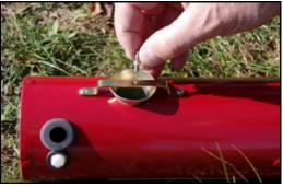
The propane nozzle will screwed into the nozzle-bracket from the sound tube.
