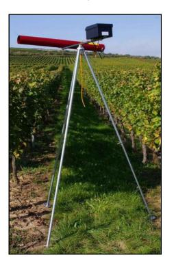
Using the adjustable pole the unit can be adjusted to the ground that the unit stands horizontally.
