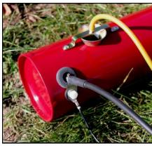
The spark plug is inserted through the opening of the rubber grommet. Then the plastic screw is screwed into the thread insert rubber and tightened firmly.
