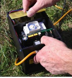
Open the lid of the electronic unit (108511) and make sure that the paper strip between the batteries and the contact board is removed.
