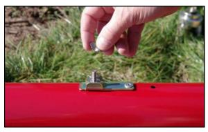
Remove the wing nut, toothed washer and the washer from the thread on the sound tube (106040).
