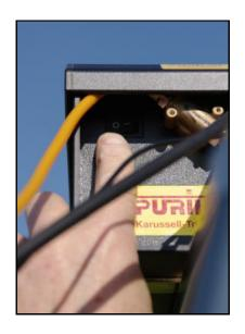
Open the valve of the gas bottle and switch on the unit.
