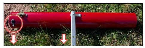
Make sure that the opening from the sound tube for the spark plug shows in the same direction like the cross bar (see picture)
