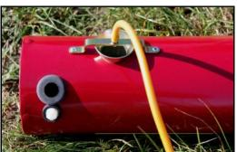
Now the gas hose is pushed onto the gas nozzle. Make sure that it is the gas hose (Gh-2) which goes away from the electronic unit.
